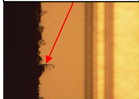
Front Side With KerfAid: 11.7 \mu m Chip Out
