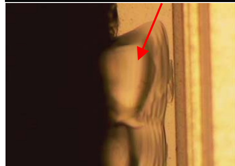
Front Side With KerfAid: 11.7 \mu m Chip Out
